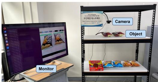
Fig. 2. Unmanned Store Testbed
